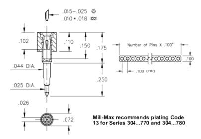
**Description:** Interconnect Socket Solderless Press-Fit Socket Accepts .015" - .025" (0,38 - 0,635 mm) dia leads Single Row Through Hole Plating Code: Shell Plating: 10 μ" Gold over 100 μ" Nickel
